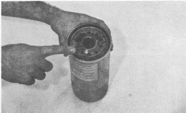
5. Coat the seals with engine oil.
